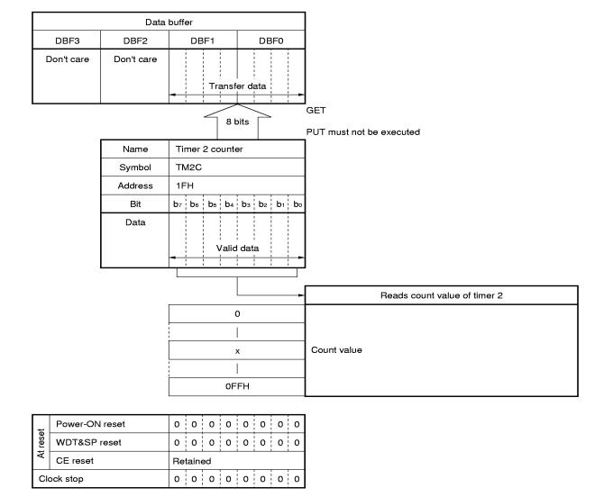
Figure 13-23. Configuration of Timer 2 Counter
