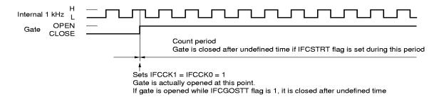
The gate is opened or closed in the following two ways when opening the gate is selected as the gate time.
