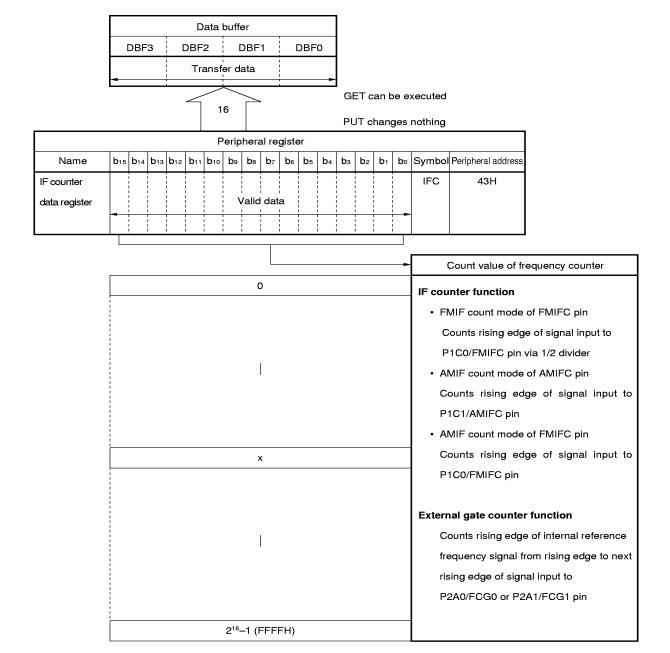
Figure 18-8. Configuration of IF Counter Data Register
