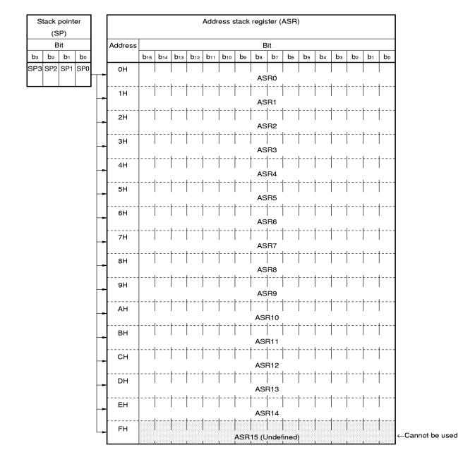
Figure 3-2. Configuration of Address Stack Register
