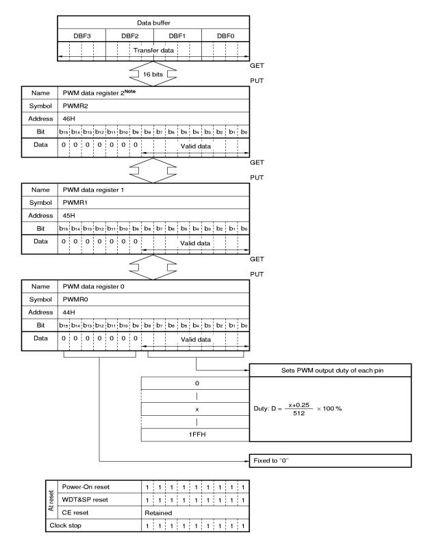
Figure 15-7. Configuration of PWM Data Registers (with 9-bit counter selected)
