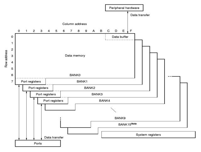
Note Port input/output selection registers are allocated to addresses 60H through 6FH of BANK 15.
