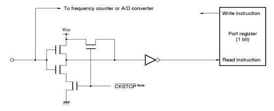
Note This is an internal signal output on execution of the clock stop instruction, and its circuit is designed not to increase the current consumption due to noise even if the pin is floated. (Except P1A3, P1A2, P1A0)
