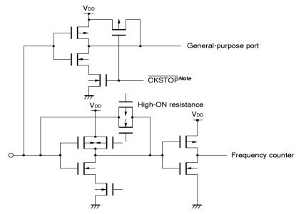
**Note** This is an internal signal output on execution of the clock stop instruction, and its circuit is designed not to increase the current consumption due to noise even if the pin is floated.
