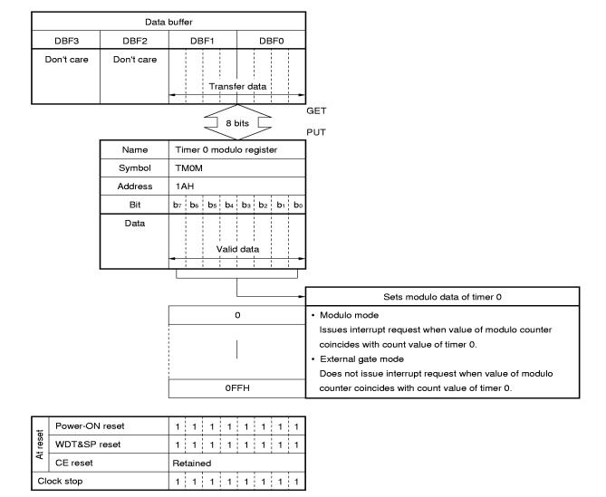
Figure 13-16. Configuration of Timer 0 Modulo Register
