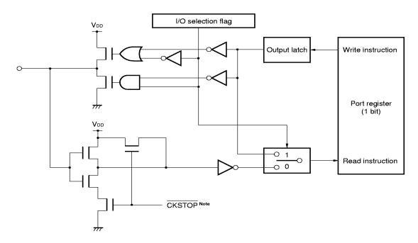
**Note** This is an internal signal that is output when the clock stop instruction is executed, and this circuit is designed not to increase the current consumption due to noise even if it is floated.
