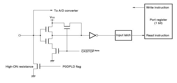
Note This is an internal signal output on execution of the clock stop instruction, and its circuit is designed not to increase the current consumption due to noise even if the pin is floated.
