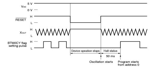
Figure 21-10. Reset Operation by RESET Pin
