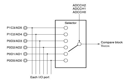
Figure 14-2. Configuration of Input Selection Block
