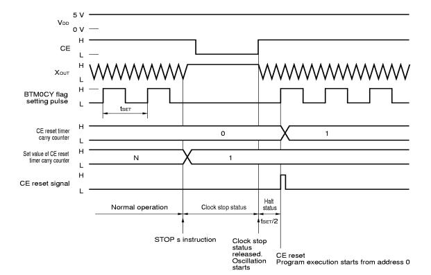
Figure 21-4. CE Reset Operation with Clock Stop Instruction
