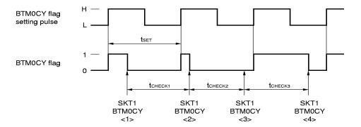
As shown in Figure 13-5, the timer is updated because BTM0CY flag is "1" when it is detected in step
