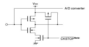
**Note** This is an internal signal output on execution of the clock stop instruction, and its circuit is designed not to increase the current consumption due to noise even if the pin is floated.
