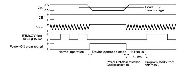
Figure 21-5. Operation of Power-ON Reset
