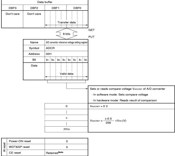
Figure 14-6. Configuration of A/D Converter Reference Voltage Setting Register
