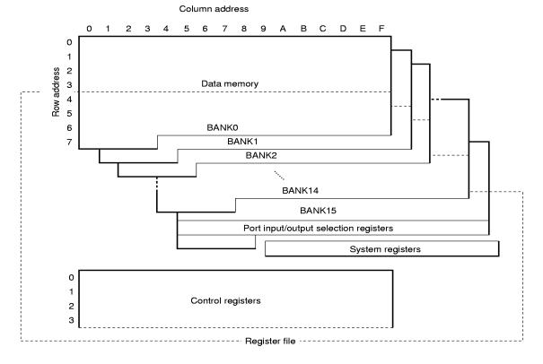
Figure 8-2. Configuration of Register File and Relationship with Data Memory
