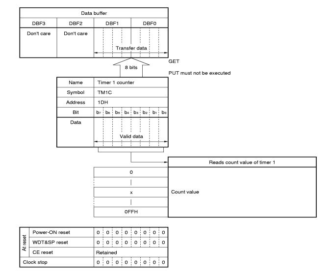
Figure 13-19. Configuration of Timer 1 Counter
