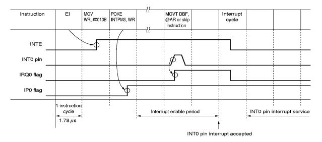
Figure 12-19. Timing Charts When Interrupt Is Accepted (2/3)
