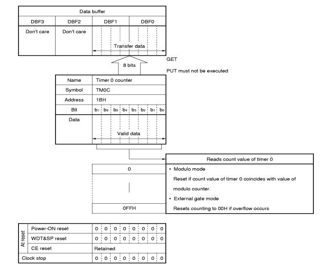
Figure 13-15. Configuration of Timer 0 Counter
