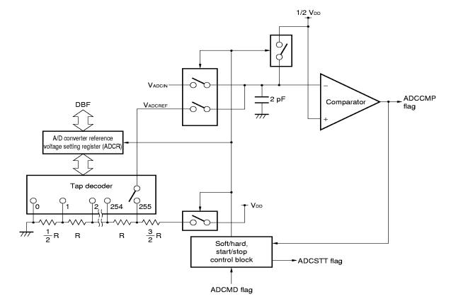
Figure 14-4. Configuration of Compare Voltage Generation and Compare Blocks
