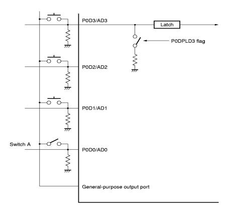
The "HALT 0001B" instruction is executed after the general-purpose output ports for key source signal are made high. Note that if an alternate switch is used as shown by switch A in the above figure, the halt status is released immediately because a high level is input to the P0D0/AD0 pin while switch A is closed.
