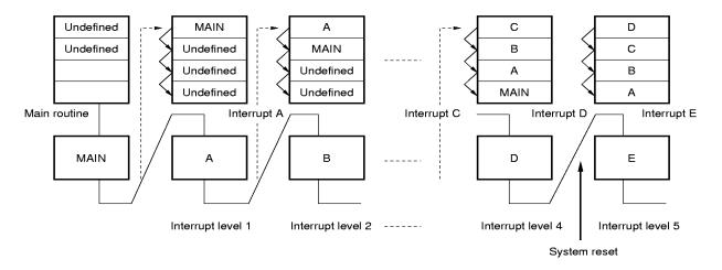
Caution The system is reset when an interrupt of level 5 is accepted.
