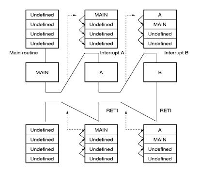
Figure 12-18. Operation of Interrupt Stack (2/2)
