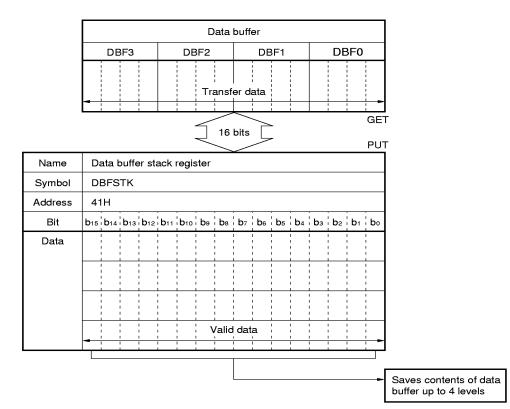
Figure 10-2. Configuration of Data Buffer Stack Register
