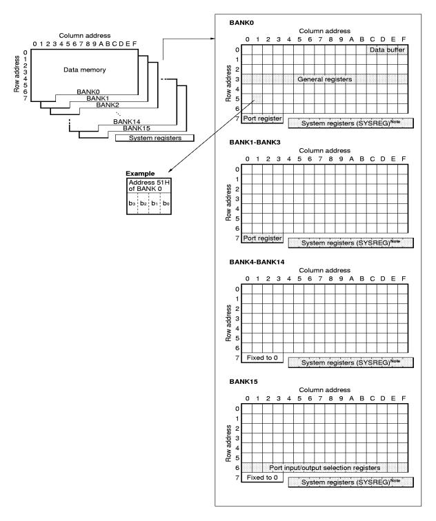
Note An identical system register exists.
