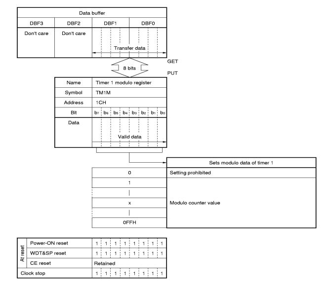
Figure 13-20. Configuration of Timer 1 Modulo Register
