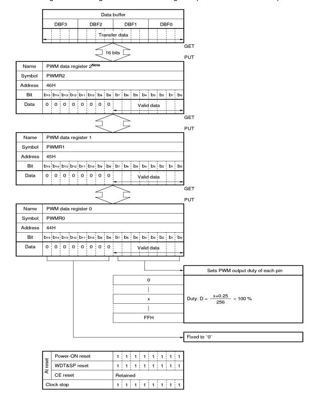
Figure 15-6. Configuration of PWM Data Registers (with 8-bit counter selected)
