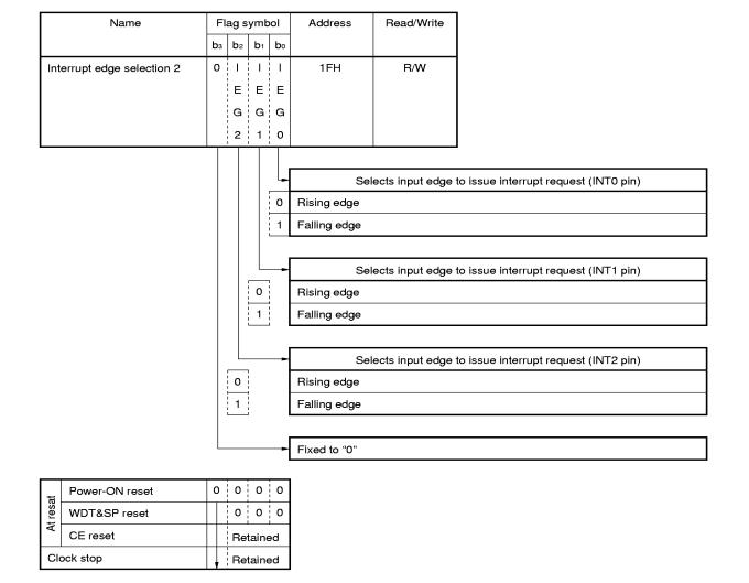
Figure 12-21. Configuration of Interrupt Edge Selection Register (2/2)
